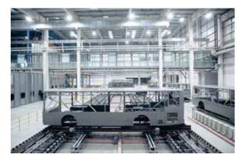
All-terrain road simulation test for whole vehicles enhances the reliability of whole vehicles and reduces the maintenance costs. The experimental standard of Yutong test track is dozens of times test strength of real vehicles. The 1,000,000km test can be completed within 30 days in Yutong's experiment center.
